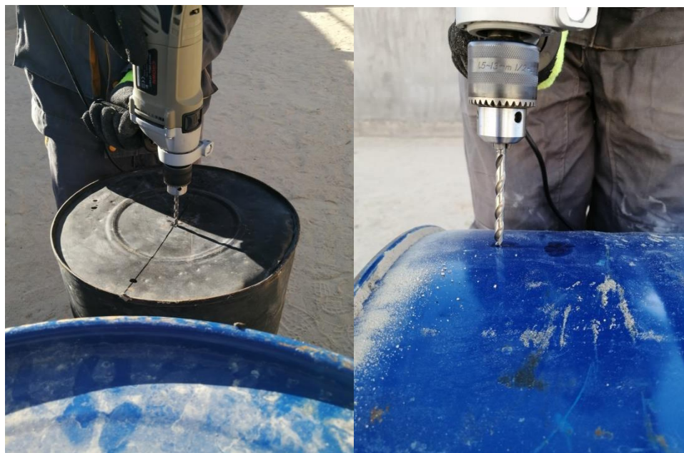
Photo02: Drums hole to enter the air.
