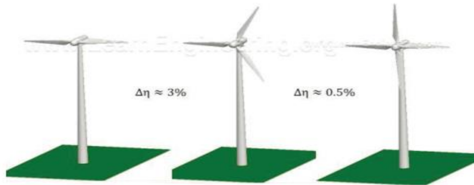
Figure.II.12. Efficiency gain increases by increases the number of blade.
