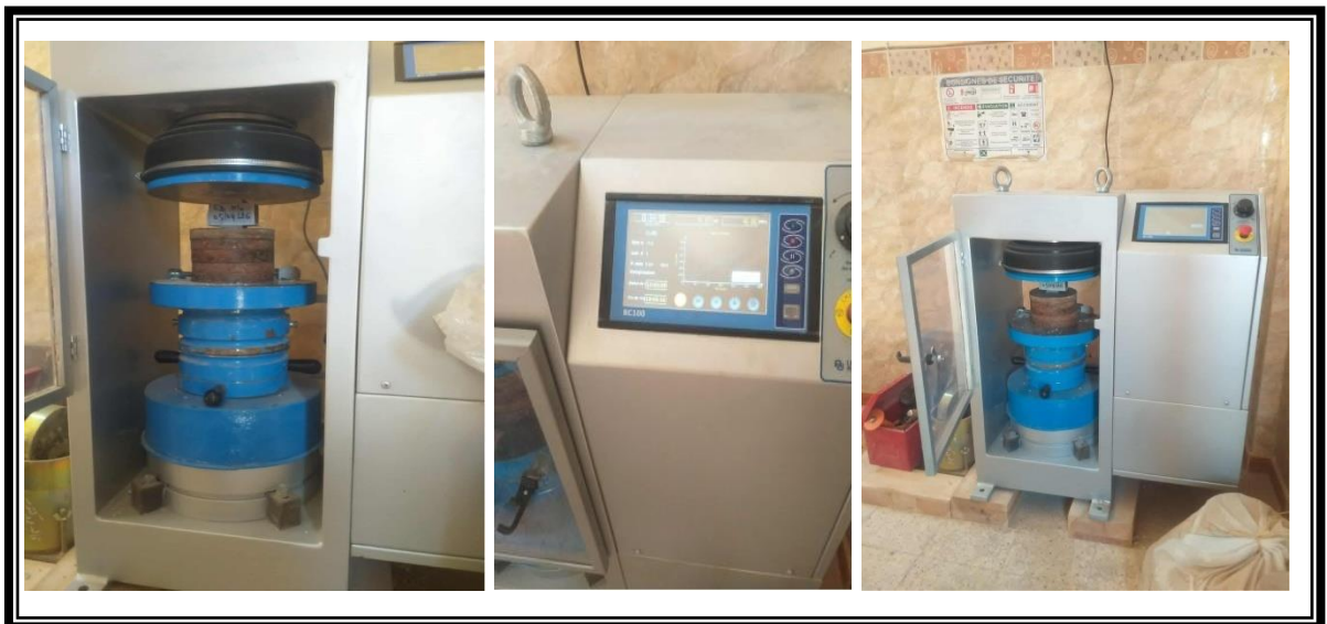
Figure II.27 : Essai de Compression
