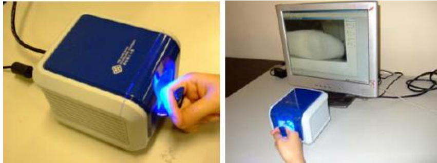
Figure 2.5: The outlook of the developed FKP image acquisition device The device is being used to collect FKP samples.
