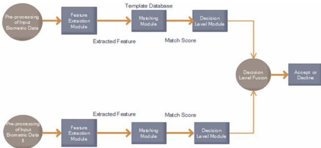
Figure 3.5: Process of Fusion at the Decision Level .
