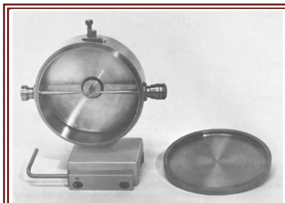
Fig. 6-1 Debye-Scherrer camera, with cover plate removed. (Courtesy of Philips Electronic Instruments, Inc.)
